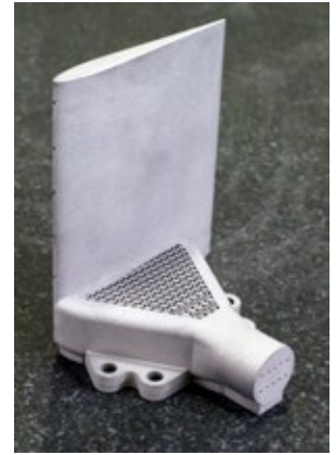
Small internal passages not possible by machining
